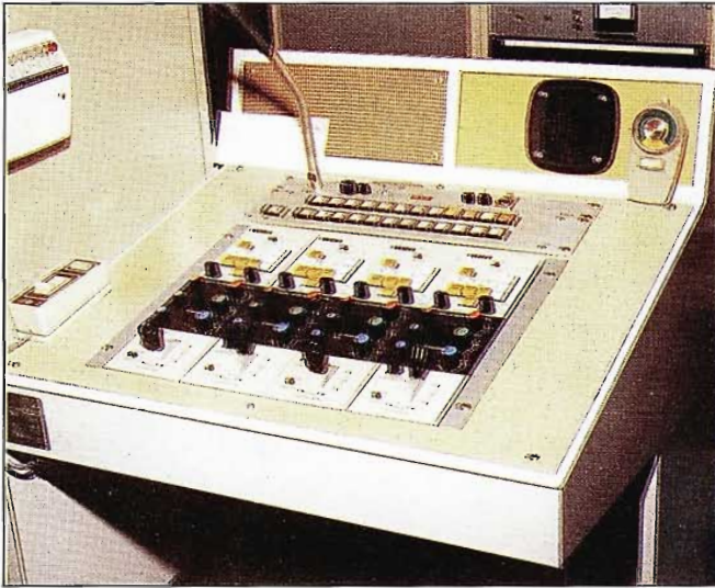
Four TK-47 Remote Control Units aboard mobile unit.
